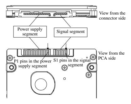
Figure 3.8 Power supply pins (CN1)
